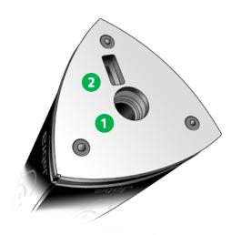
Jabra Noise Guide has 2 inputs at the bottom of the device.
