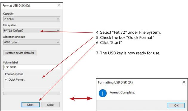
**WE RECOMMEND** that you format the USB memory stick before either reading log data from the internal memory of the Jabra Noise Guide to the USB memory stick, or transferring a new configuration by USB to the Jabra Noise Guide.
