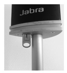
1. Face the Noise Guide, so you have the USB port on the left from the tube.
